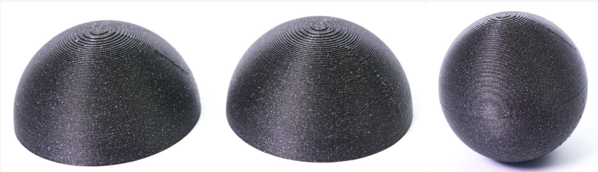
Printing a sphere cut into two hemispheres, which are then glued together.
